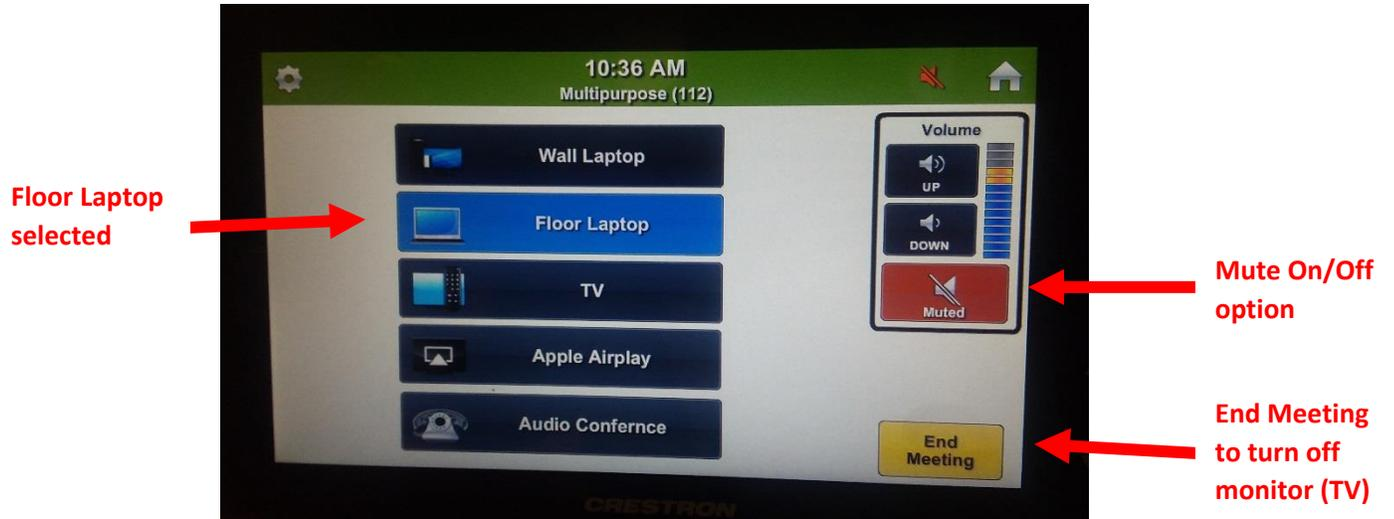
Furthermore, to make telephone calls select the **“Audio Conference”** option at the bottom of the Crestron Tablet and a number pad will be displayed for you to enter the phone number.
